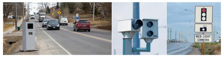
PHOTOS (Left to right): 01 Automated Speed Enforcement camera on side of road | 02 A red light camera | 03 A red light camera road sign
