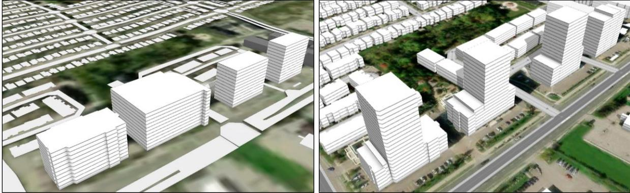
Figure 7: Level of Detail Comparison - Single Height Attribute vs, Delineated Heights
