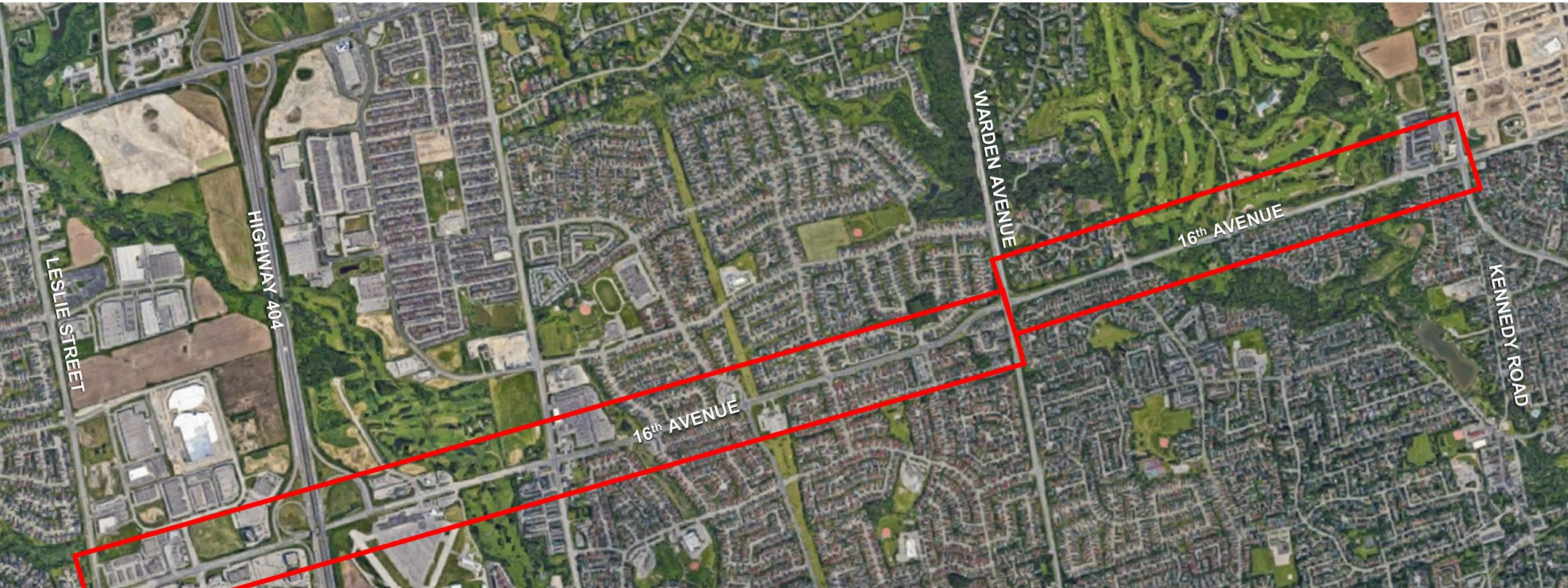
Road widening from four to six lanes, widening of the Highway 404 bridge, rehabilitation of Rouge River bridge, active transportation, sidewalk, illumination and streetscaping
