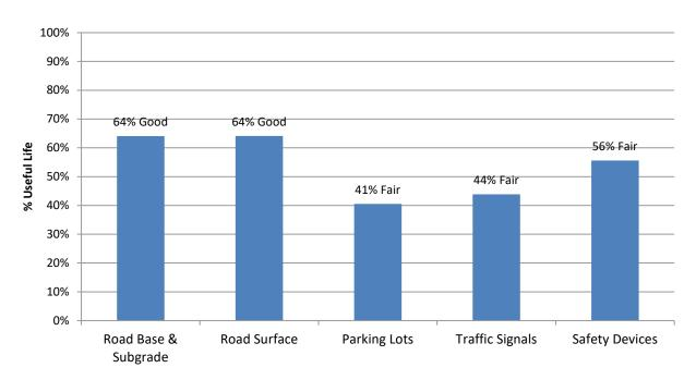
Figure 3-18: % Remaining Useful Life by Component and Condition Rating – Roads
