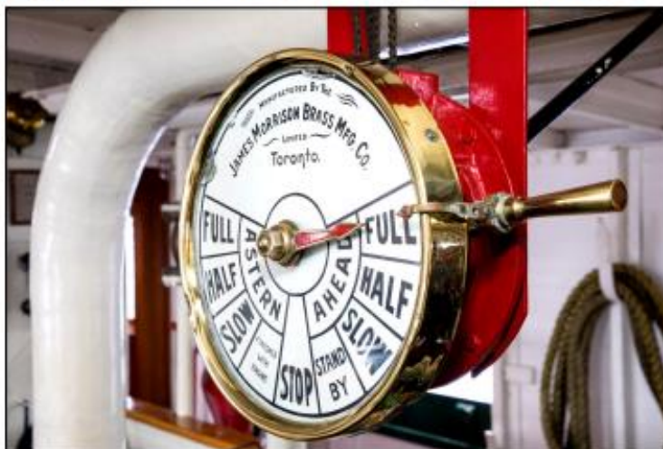
Telegraph on board the RMS Segwun, the oldest operating steamship in North America. (Photo courtesy the Town of Gravenhurst)
