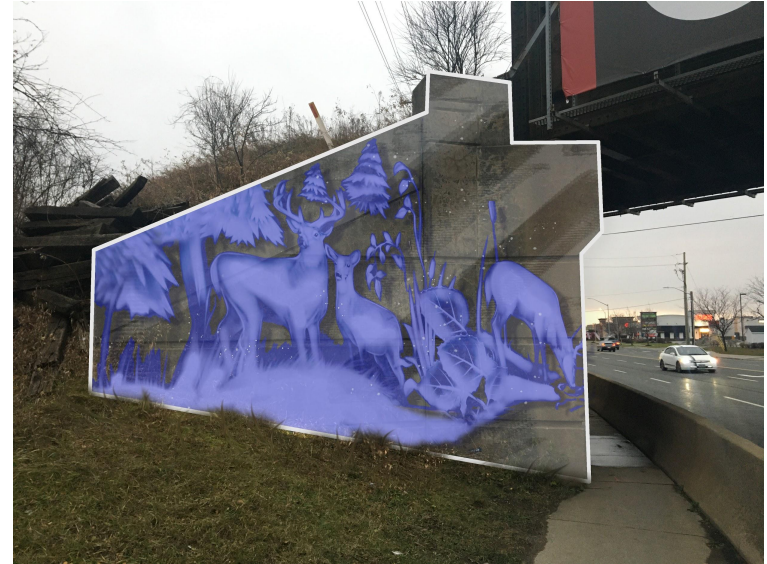
Etched glass can be edge lit using RGB LEDs creating a variety of colour
