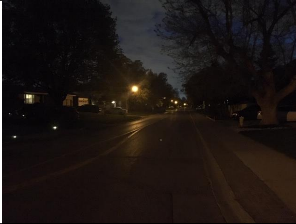
EXISTING: Fred Varley Dr with Decorative HPS Do not meet minimum Lighting Levels
