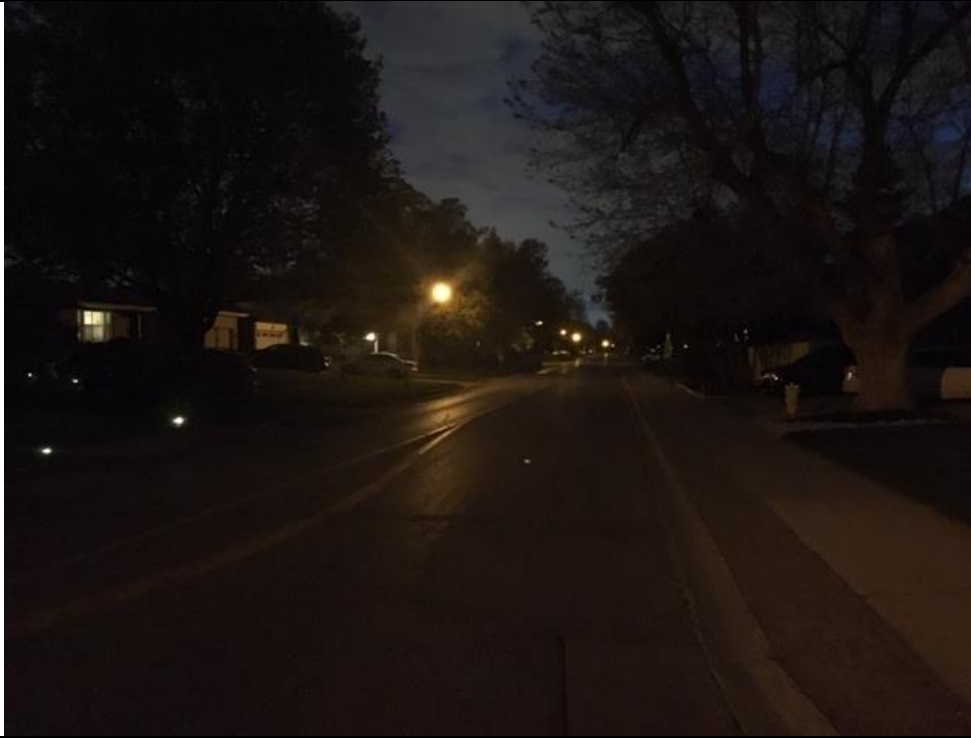
EXISTING: Fred Varley Dr with Decorative HPS Do not meet minimum Lighting Levels
