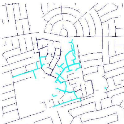
Figure 3: Pipe Missing Elevation with Both Ends
