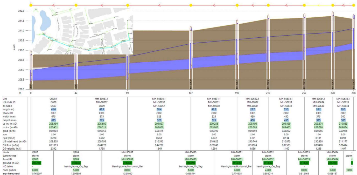
Figure 36: 100 Yr HGL Level – Pipes Upstream to East Pond South Inlet – Base Scenario
