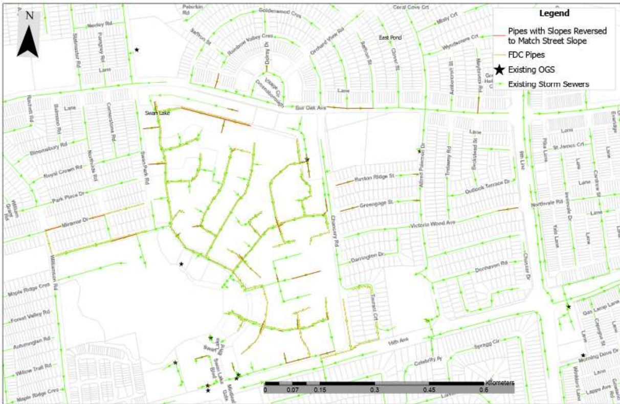
Figure 6: Pipes with Slope Reversed to Street Slope
