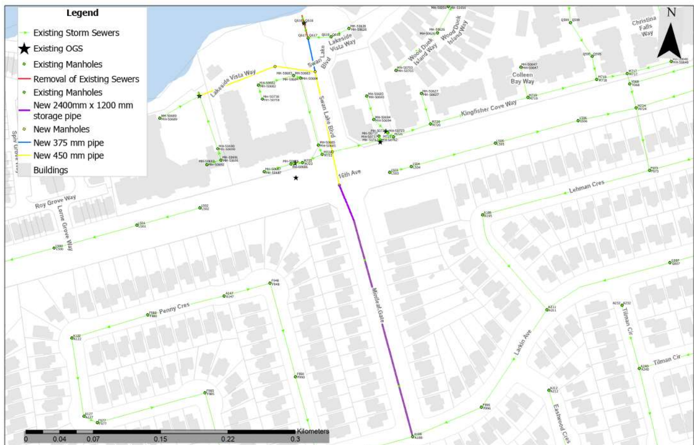
Figure 38: System Upgrade Requirement to Achieve Scenario 7 (Box Storage Implementation on Mintleaf Gate)
